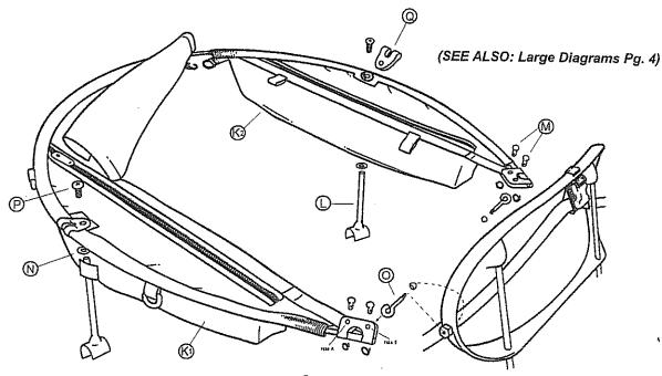
**STEP 4-** Grasp K1 with zipper facing up and insert eyebolt on left side of seatback into hinge and align with hole B. Secure eyebolt to hinge with clevis pin and split ring. Repeat procedure with K2, securing hinge to eyebolt on right side of seatback with clevis pin and split ring.
