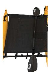
Another feature are the forward bungee straps for securing the trampolines while not in use. To use them unbuckle the rear of the trampoline, roll the material up toward the forward AKA and wrap the bungee around and onto the hook.
