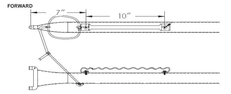
The paddle shaft will snap into the holder located at the rear aka, at the hinge point of the aka brace.
