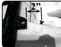
2. Install the dodger onto the kayak with the mast installed as it would be when sailing. There are clips on the front and forward edges to allow you to install the dodger without having to remove the mast or deck mounted bars.
