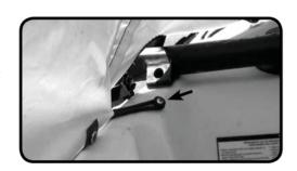
3. To hold the dodger tighter against the side of the kayak, snaps have been attached to the edges of the dodger. To snap these to the hull, you will need to bolt the snaps included in this kit to the side of the kayak. Use the snap locations on the dodger as a guide of where to install the snaps onto the hull. Use the washer and nut to through bolt the snap to the kayak.
