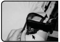
There is a small loop of line that is sewn to the inside front corner of the dodger. Loop this line over the eyelet post that was installed in step one.
