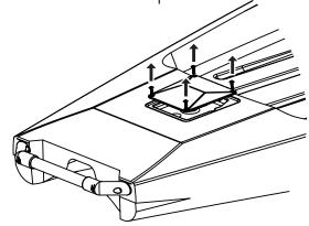
(3) Align the clamps around the rear handle & install the 10-32 screws, washers & nuts. Add shims & longer screws for PA12. **Do not tighten.**
