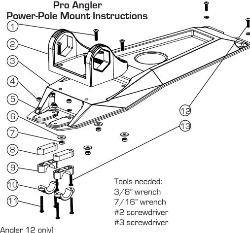
1 Assemble Power-Pole base to Hobie Power-Pole mount using 1/4" screws, washers & nuts.
