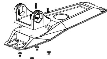
(2) Remove screws & rudder cover. Save screws for next step.
