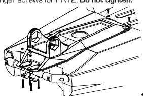
4 Using the #10 washers and the #10-32X3/4 screws from the rudder cover fasten the front of the mount.
