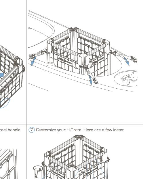
6 To secure rods, pull bungie handle over reel handle and secure in slot next to pad eye.
