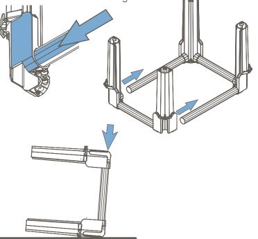
(3) Align the bottom of the crate. To secure it, first push in the centers of the walls to clear the center snaps and install the thread forming screws in the corners. (optional) To add extra ridgitiy, you may install the self tapping screws into the holes on top of the corners
