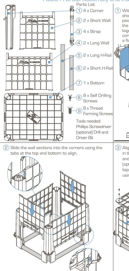
With the flat surfaces aligned, insert 2 long and 1 short H-Rail section into two upside down corner pieces. Then connect the remaining corners using the short H-Rail segment sliding both assemblies together. Ensure the rails go all the way into the corners. You may need to push them together using a flat surface for leverage.
