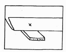
Fold material for hem, mark for hole, and place wood block beneath material.
