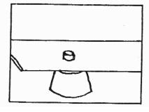
Insert grommet (D) thru hole. Set firmly on base (C) line up hole in grommet with hole in base.
