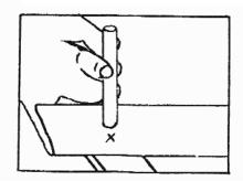
Place cutter (A) over mark and strike with hammer to make holes.
