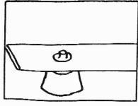
Insert point of die (B) into tube. Strike lightly with hammer turning die slightly between blows until the two haves fit tightly together.
