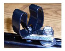
3) Place the desired tiller grip sized fitting onto the assembly and slide over the "T" lock bolt with the tiller grip's bolt in the track, or to one side, to obtain the proper angle for the tiller. Tighten the tiller grip bolt / nut. Tighten the "T" lock bolt / nut to hold in the desired position. Repeat for opposite side.
