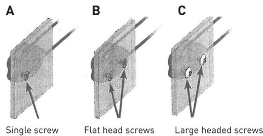
If you only have one screw holding the block **(A)**, an additional hole will need to be drilled to bolt through another location. To drill a new hole, locate the single screw currently holding the block and drill a 3/16" hole 1-1/8" back from the center of the current screw. This will allow the new hole to align with the other bolting location on the block.
