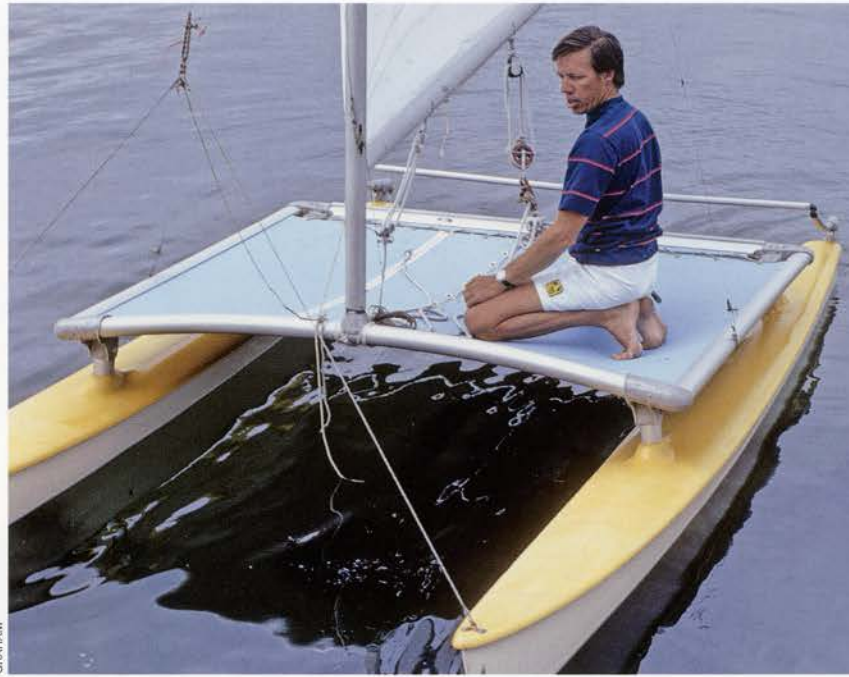
Hobie aboard the 16': "Kick-up rudders, controllable by the skipper from the tramp, no dagger boards, one sheet line, then one guy could single-hand it from the beach and have some fun." Circa 1972.
