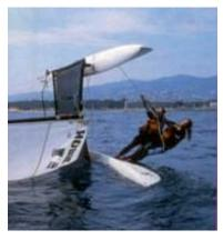
If you tip the boat over, in order to avoid the mast from sinking under the hull, one of the crew must rapidly climb on the hull that remains on the water. In the meantime, the other crew uncleat all the lines and sheets.
