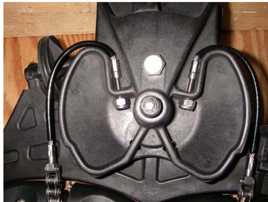
6A. Insert idler cable into rear slot as shown. Note -- this slot is divided -- use outboard portion of slot (left).
