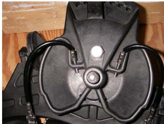
5A. Slip cables over top lip and hand tighten new Nyloc nuts to keep cable from slipping out (right).
