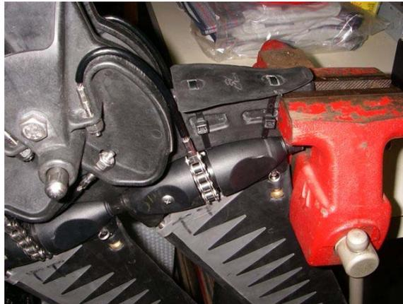
4 B. Mount both drum / crank arm assemblies to drum shaft, noting correct left and right side.
