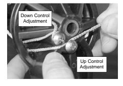
If the up-line still does not reach the control arm, you can let some slack out on the up-line by loosening the up-line screw on the rudder housing. There are two screws on the rudder housing next to the center axle. The up-line will feel slack, and you can loosen the screw to pull some slack through the rudder drum. You may also need to adjust this screw if there is too much slack in the line.
