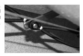
5) At the stern, locate the up-line running to the rudder. It is one of the two center lines running to the rudder, and it should be slack.
