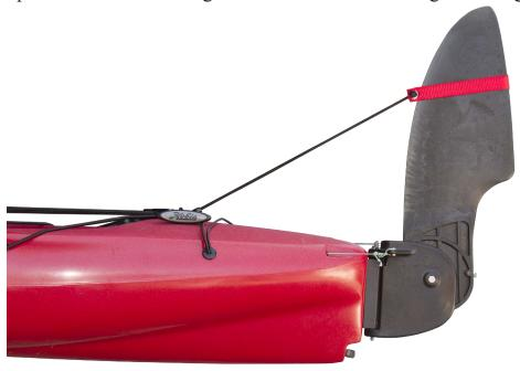
(2) Rudder pin removed and stored horizontally: Remove the rudder pin by first removing the key ring at the bottom of the pin and then lifting the up/down control lines over the top of the pin so that the pin can be pushed up from below and fully removed. Remove the rudder from the gudgeon, then replace the pin in the rudder and secure with the key ring. Rotate the rudder horizontally and secure it to the hull using the Bungee® that is attached to the hull.
