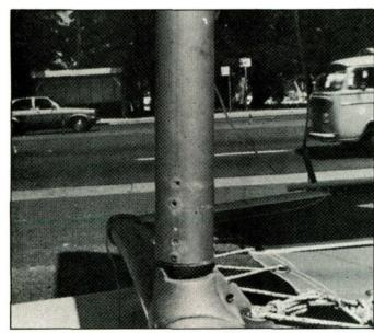
Straight line extended through fore and aft axis of mast extrusion should line up between front corner casting and sidestay chainplate.
