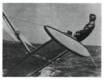
(2) In puffs or in steady, high-wind conditions, while the jib contributes little to the performance of the boat on a close reach or going to weather, in fact as I mentioned above, it seems to be detrimental. It does definitely produce a greater tendency for the Hobie Cat 14 to "bury the leeward bow." This is in contradiction to the claim that the jib has a tendency to lift the bows.
