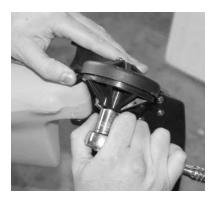
If the rudder still sticks after you remove and change the up control bungee, loosen the hex head bolt a little bit. Do not make complete turns with the bolt, the slightest adjustment can make a big difference.
