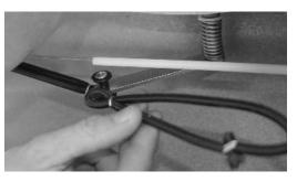
3) There are two bungees attached to the up/down control arm, looped around eyelet posts
