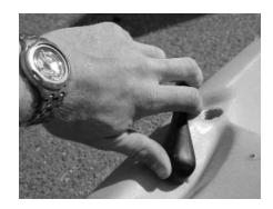
If the up-line will not reach the eyelet post, rotate the rudder up-down handle slightly (the handle on the outside of the boat) with your other hand to bring the control arm closer to the line.
