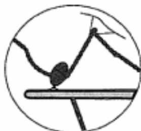
H-18sx H-215E Rivet eye strap to outboard end of wing tube. Shackle block to eye strap. Twist on spring as though putting key on key ring. Spring holds block in upright position.
