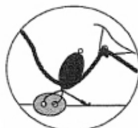
H-20 Tie line through rear crossbar end cap and around bolt, fasten to block. Hook bungee to trampoline lace line to hold block from water.
