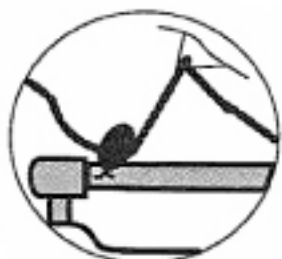
H-16 Rivet eye strap to rear end of side bar. Shackle block to eye strap. Twist on spring as though putting key on key ring. Spring holds block in upright position.
