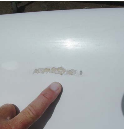
A three-inch gouge on the hull of a Hobie 16
